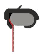
STEP 2: ROTATE CLIP COUNTERCLOCKWISE
